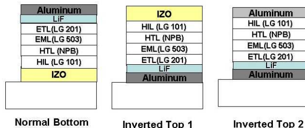
Figure 1. Device structures of normal and inverted OLEDs.
