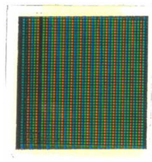
Figure 9. A 2"x2", 22 dot-per-inch color-pixelated CLCD.
