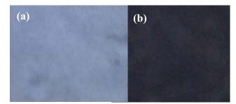
Fig. 2. Photomicrographs of the black/white electrophoretic ink suspension cell in power-on state. (a) is +10V applied on the front electrode, and (b) is -10V applied on the front electrode.
