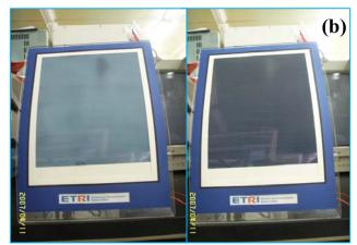
Fig. 3. Photographs of A4-sized electronic ink panel with an electrophoretic ink microcapsule diameter 50  $\pm$  10  $\mu$ m in power-on state.
