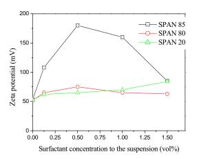
Fig. 1. Zeta potential of TiO<sub>2</sub>/PS electrophoretic particle suspension with three different surfactants.
