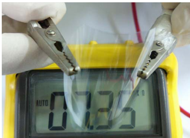
Fig. 3. Clear and homogeneous t-MWNTs network.
