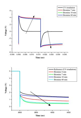
Fig. 4. The changes of VHR (%) and RDC (V) of LC cell after interfacial reacted with bromine.
