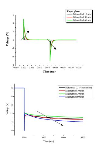
Fig. 3. The changes of VHR (%) and RDC (V) of LC cell after interfacial reacted with ethanethiol.
