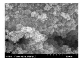
Fig. 4. SEM image of SnO<sub>2</sub> fillers used to fabricate the CNT paste.
