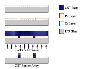
Fig. 2. Schematic fabrication processes of dotpatterned CNT emitter arrays by using photosensitive CNT paste.
