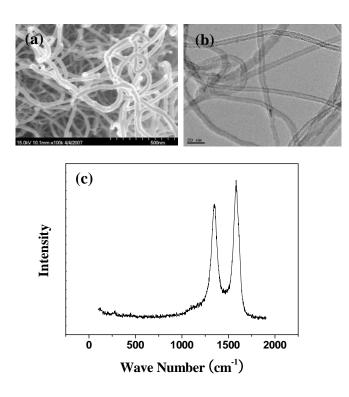
Fig. 1. (a) SEM and (b) TEM images and (c) Raman spectrum of CNTs used to fabricate the CNT paste.
