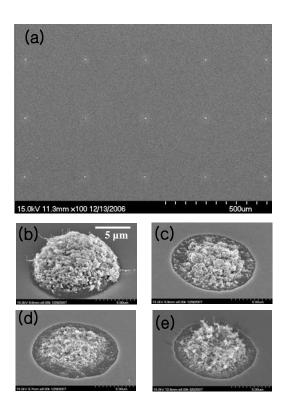
Fig. 3. SEM images of 10-µm-diameter dot arrays patterned by using the photo-sensitive CNT paste: (a) an array of CNT paste dots, (b) a dot after developing, (c) a dot after firing, (d) a dot after tape activation, and (e) a dot after measuring field emission.
