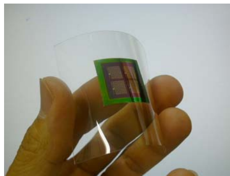
Fig. 6. Transferred poly-Si TFTs on PES substrate.
