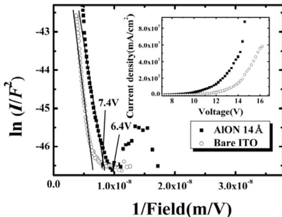
Fig. 4. Fowler-Nordheim tunneling plot with (a) and without (b) AION treatment of the ITO surface. The curve in the close up shows the current density-voltage ( $J$ - $V$ ) properties of the devices
