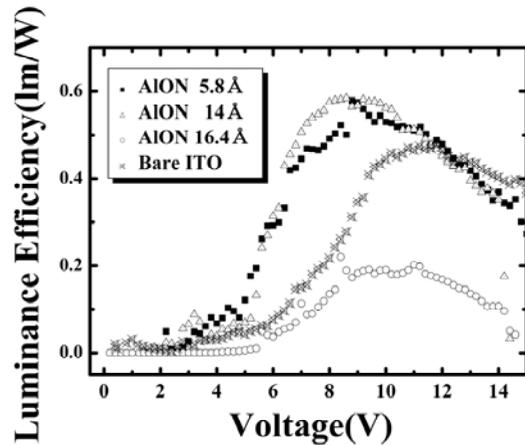
Fig. 3. Luminance efficiency-voltage characteristics without and with buffer layer
