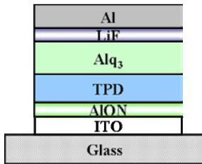
Fig. 1. The device structure of OLEDs with AION buffer layer
