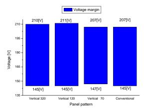
Fig. 5. Voltage margin characteristics for the conventional and IBS electrode structure panels.
