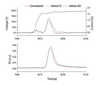
Fig. 9. Discharge currents and waveforms for the conventional and IBS electrode structure panels.
