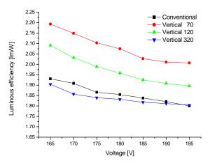
Fig. 8. Luminous efficiency for the conventional and IBS electrode structure panels.
