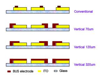
Fig. 4. Schematic drawing of conventional and IBS electrode structure with the vertical length of 70, 120, 320um respectively
