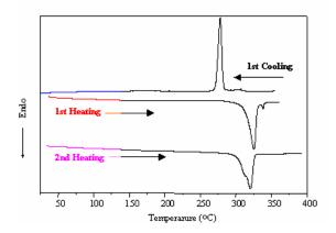
Fig 2. DSC Thermograms of compound with R=H (Heating and cooling rates =  $10^{\circ}$ C/min).
