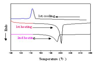
Fig 4. DSC Thermograms of compound with  $R = OC_8H_{17}$  (Heating and cooling rates = 10°C/min).
