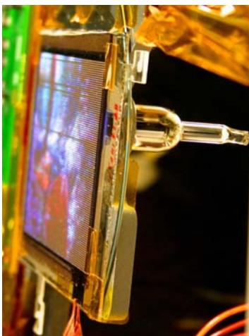
Figure 4. View of CNT FED with Pinch Off Tube and 50% Neutral Density Filter
