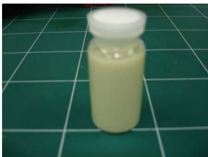
Fig. 4. ITO ink formulated using ultrafine ITO nanoparticle.
