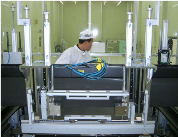
Fig. 3. Developed precise screen printer for color filter printing.
