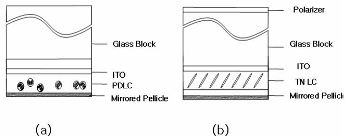
Fig.1. The cross sectional structure of PDLC modulator (a) and TN modulator (b).
