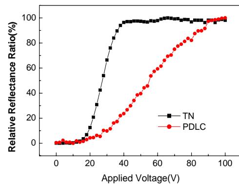
**Fig. 4. The electro-optic characteristics of TN modulator and PDLC modulator.**
