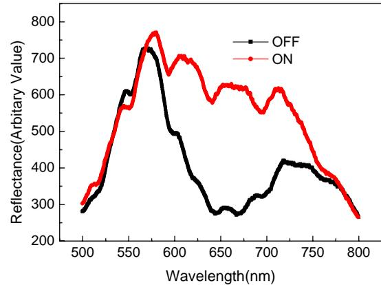
**Fig. 3. The measured on/off reflectance curve of the TN modulator.**
