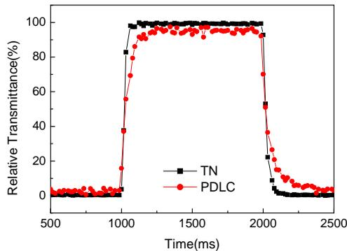
**Fig. 4. The response characteristics of TN and PDLC modulators.**
