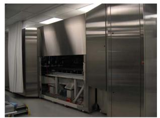
Fig. 1. Gen 7 LCD Color Filter Machine developed by Kodak for DuPont TCF Process.
