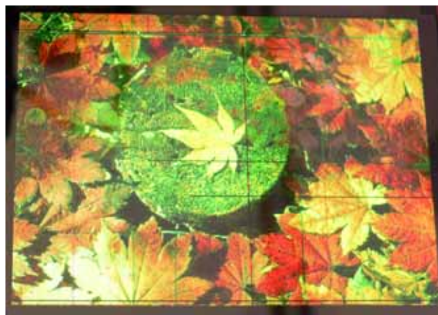
Fig. 6. AMOLED display driven by GaInZnO TFT
