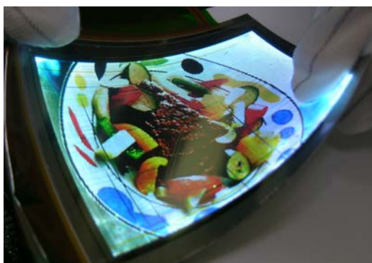
Fig. 5. 3.5 inch full color QCIF + AM-OLED panel on a metal substrate
