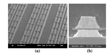
Fig. 3. SEM Images of aluminum electrode after chemical etching steps: (a) top and (b) cross sectional view
