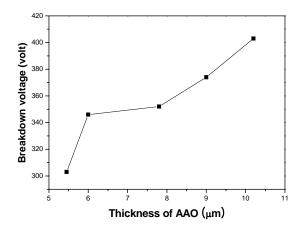
Fig. 5. Effect of AAO thickness on the breakdown voltage of AAO dielectric layer.
