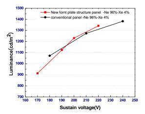
Fig.8. Luminance of test panels with anodic aluminum oxide layer. The luminance of conventional test panel using Ag electrode with glass dielectric layer is also shown in the figure for comparison.
