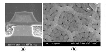
Fig. 4. SEM images of anodized aluminum electrode: (a) cross sectional and (b) surface view.
