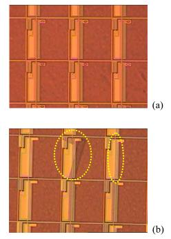
Fig. 3. Microscope images of the pentacene islands formed by (a) PC-OVD and (b) a conventional thermal evaporator.
