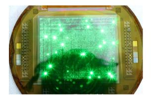
Fig. 4. An Image of the 3.5 inch OTFT-driven OLED with green emission.
