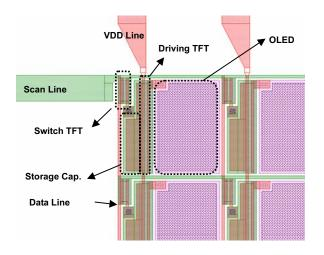
Fig. 1. Schematic Diagram of the pixel structure.
