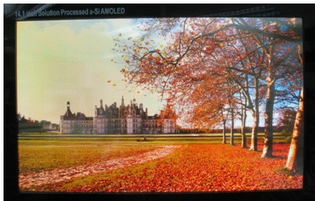
Fig. 1. Photography of SEC's 14.1 inch WXGA AMOLED Panel fabricated by ink-jet printing. It was demonstrated on 2004.
