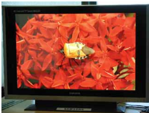
Fig. 2. Photography of SEC's 40-inch AMOLED Panel fabricated with white & color filter approach. It was demonstrated on 2005.
