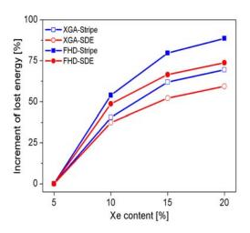
Fig. 5. Incremental ratio of lost particle energy dependence on Xe content with varying resolution and subpixel type
