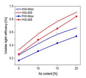
Fig. 4. Visible light efficacy dependence on Xe content with varying resolution and subpixel type
