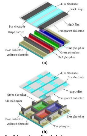
Fig. 3. Schematics of subpixel arrangement (a) Conventional structure with stripe barrier ribs (b) SDE structure
