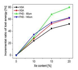
Fig. 2 Incremental ratio of lost particle energy dependence on Xe content with varying resolution
