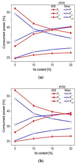
Fig. 6. Consumed power in Stripe and SDE structures as a function of the Xe content (a) XGA (b) Full HD
