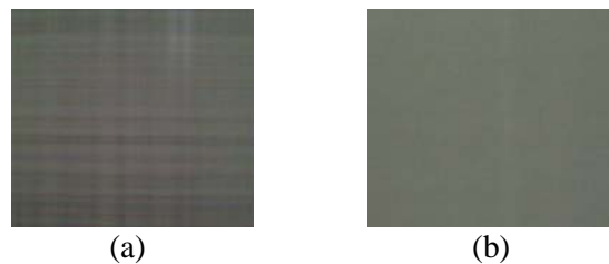
Figure 4. AMOLED display images with the pulse extension of (a) 1X (b) 4X.
