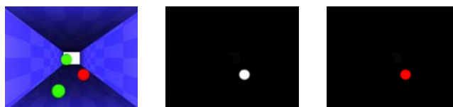
(a) Input image (b) Saliency map (c) Focus of attention Fig. 1 Schematic diagram represents the proposed attention system based on bottom-up approach.
