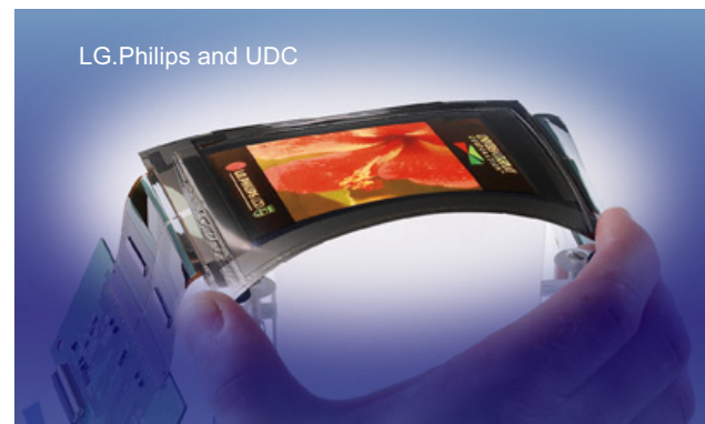
Fig 3. Flexible AM Matrix Display by LG.Philips and UDC on metal foil substrate, encapsulated with Vitex Barix encapsulation.
