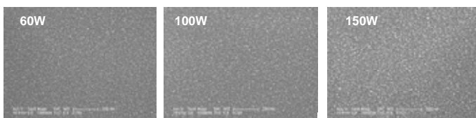
Fig. 2. SEM Images of ZnO films grown on the \text{SiO}_2 coated glass at various plasma powers.
