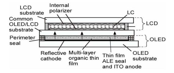
Fig. 1: Three substrate LCD/OLED integrated structure
