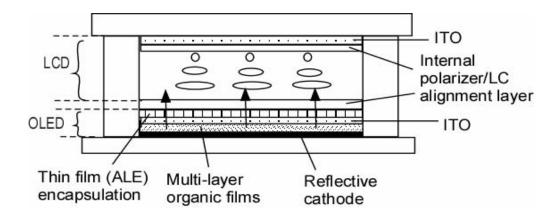
Fig. 2: OLED backlight inside LCD
