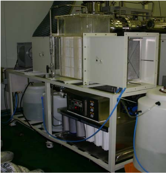
Fig. 2 Test facility for Air washer system
