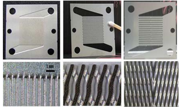
Fig. 2 The photos of straight and Y, V-shaped channel in metal sheet.
