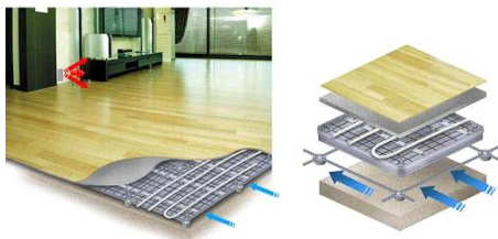
(b) Air flow into the bottom space of the multi-functional floor heating system
