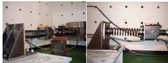
**Fig. 5** A MTS machine for the horizontal dynamic test
