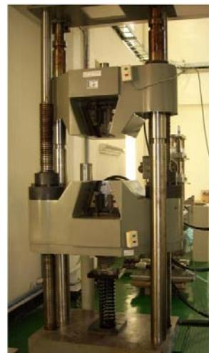
**Fig. 1** Material tester measuring spring characteristics
