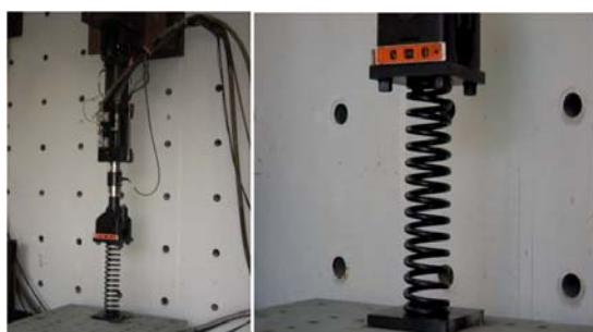
**Fig. 4** A MTS machine for the vertical dynamic test
