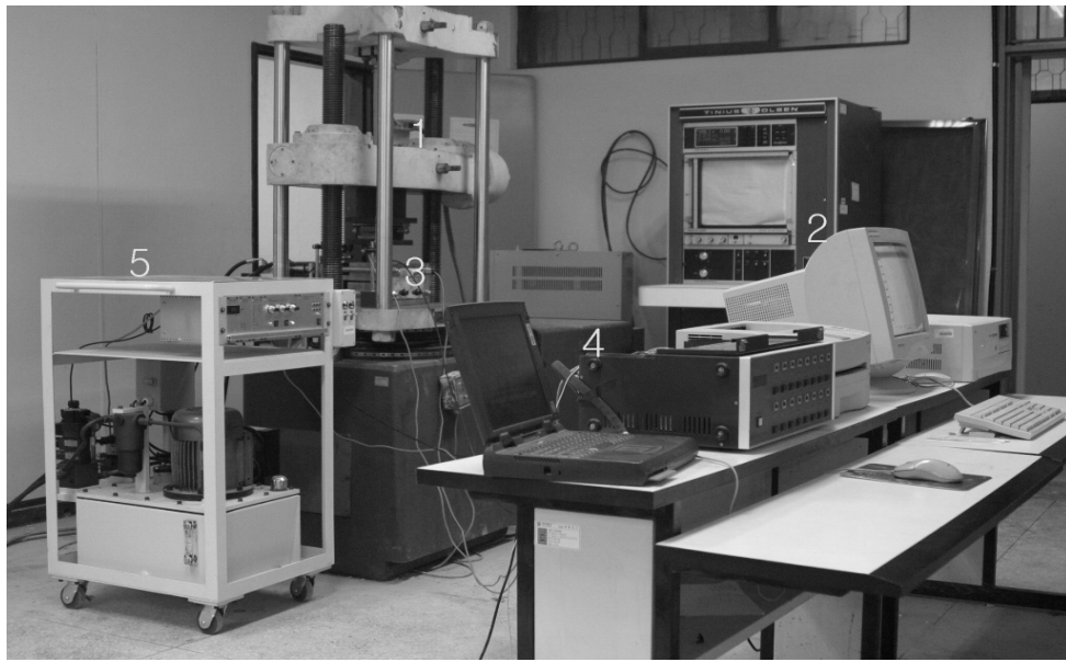
(1) UTM (2) UTM controller (3) Shear testing apparatus (4) Data acquisition apparatus (5) Shear pump
