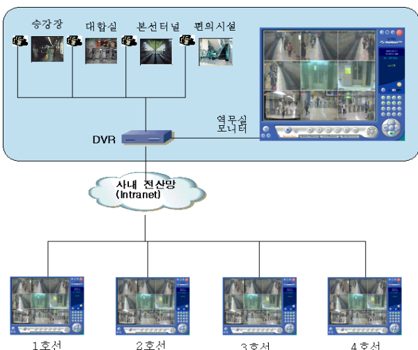
Fig. 4 CCTV recording equipment
