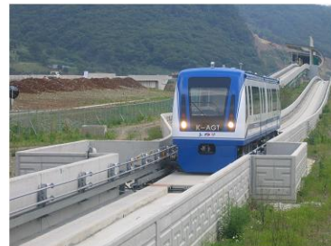
Fig. 2 Prototype (2 car-train) of the Korean-standardized rubber-tired light rail vehicle (K-AGT)
