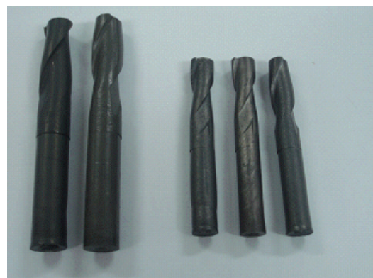
Fig. 4 Size comparison of injected and sintered endmill
