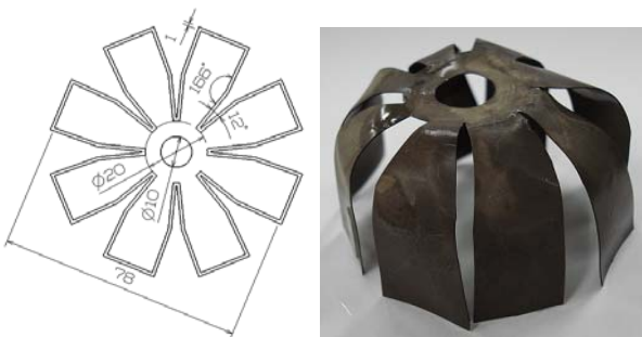
Fig. 2 Schematic of jellyfish robot
