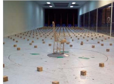
Fig. 1 The container crane model for wind tunnel test
