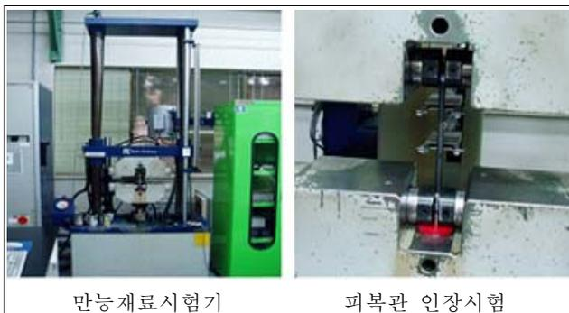
Fig 6. Universal testing machine and Test Process.
