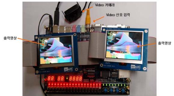
Fig. 5 Test result of FPGA IP
