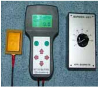
Fig. 1 Water absorption detector(Gen-SWAD I)
