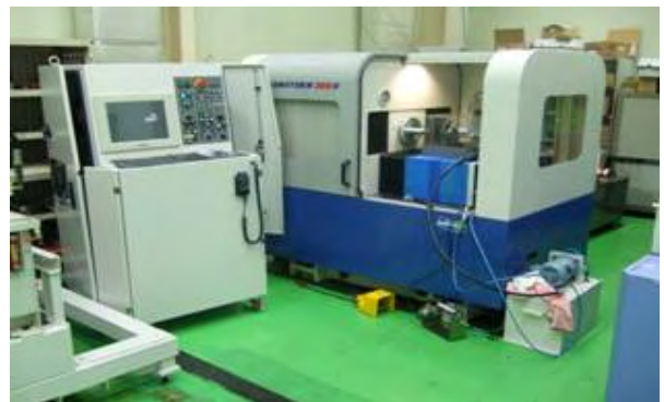
Fig. 3 Grinding machine for spheric mold core (Doosaninfracore Co., NANOTURN 300U)
