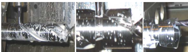
Fig. 7 5-axis machining for the step cutter
