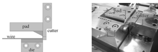
(a) schematic of shearing (b) shearing system Fig. 1 Photograph of shearing
