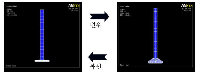
Fig. 2 Deformation Shape of Ultrasonic Linear Actuator
