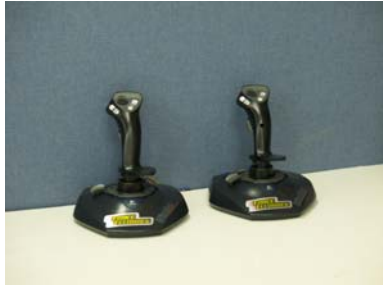
Fig. 4 Force-feedback joystick of intuitive OCU
