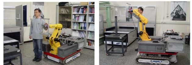
Fig. 2 Experiment for installing construction materials
