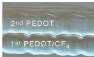
Fig. 2 Self-Aligned Printing (SAP) process and its result
