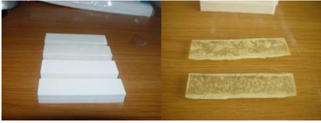
Fig. 4 Test specimens of general 3D printing (left) and UV curing (right)
