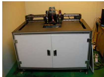
Fig. 9 8 heads UV curing system
