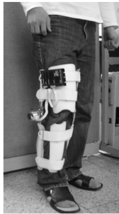
Fig. 1 Exoskeleton which can support human gait motion
