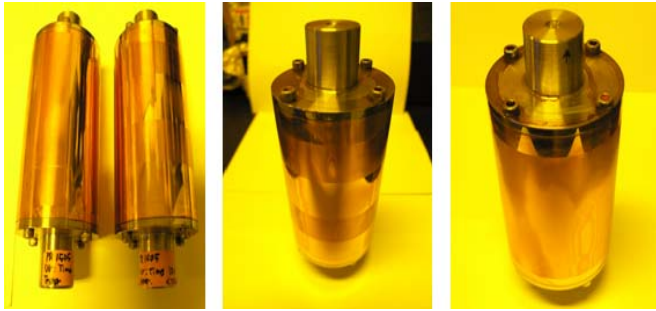
Fig. 2 Result of fabrication for high-resolution micropatterned-roll with 20 \mu m and 10 \mu m
