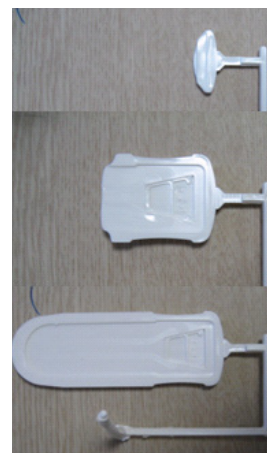
Fig. 6 Result of short shot and injection molding for the presented protein chip model
