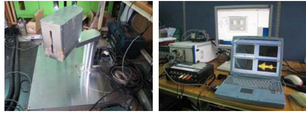
Fig. 4 3 vibration measurement of 3 axis-SCARA robot
